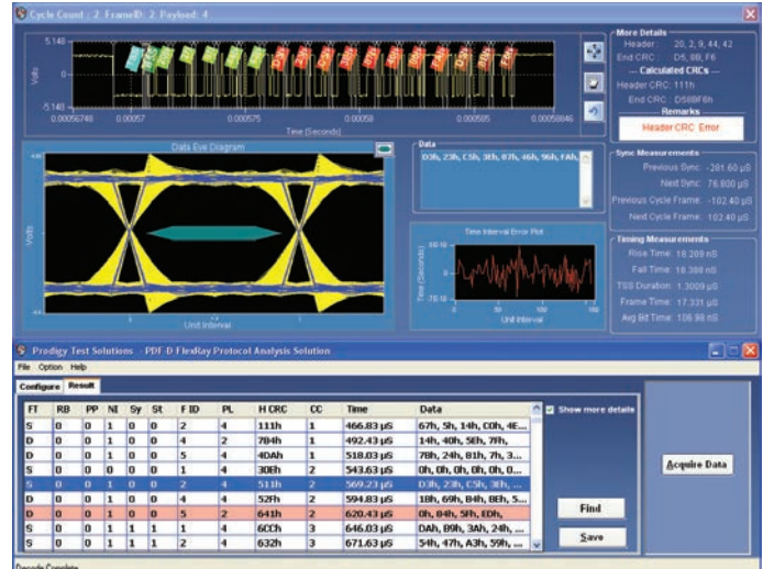
Figure 44. DPO4AUTOMAX Eye Diagram analysis of a FlexRay signal.
