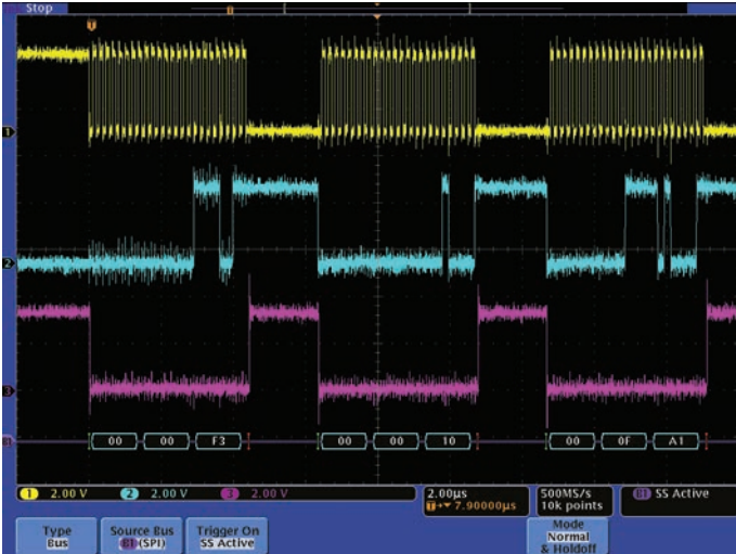
Figure 13. Correct synthesizer configuration messages.
