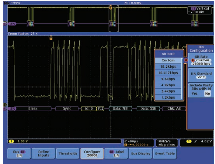
Figure 35. LIN bus setup menu and decoded frame.
