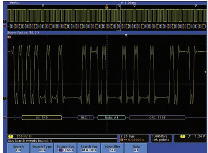
Figure 45. Searching on specified identifier and Data in a CAN bus acquisition.
