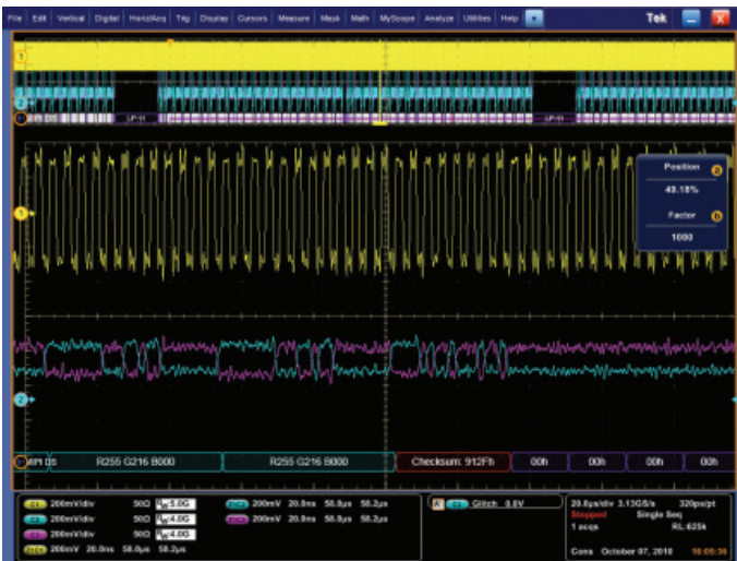
Figure 54. MSO70000C analog-channel decoded display of a Packed Pixel Stream, showing a checksum error.
